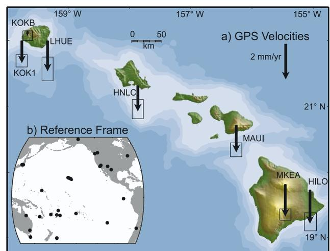
**Figure 2.** a) Vertical velocities at Hawaiian CGPS stations relative to b) the 30 CGPS stations used to establish a Pacific fixed reference frame. HNLC is located at the Honolulu Harbor tide gauge station; HILO is 500 m from the Hilo Harbor tide gauge station. 95% confidence intervals are given.
