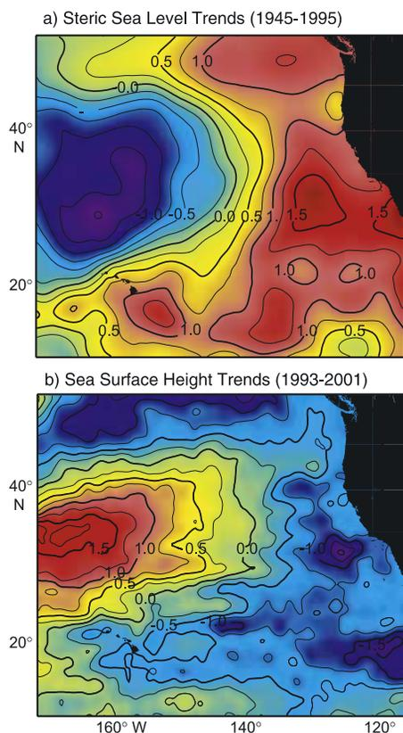
**Figure 3.** Linear trend in a) steric sea level relative to 500 m computed from the WOA gridded product (1945–1995), mm/yr, and b) sea surface height from TOPEX/Poseidon satellite altimeter data (1993–2002), cm/yr.
