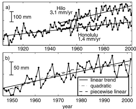
**Figure 1.** a) Annual mean sea level from the Honolulu and Hilo tide gauges, and b) the difference between the Hilo and Honolulu records. Least squares regression is used to determine linear (1.8 mm/yr), quadratic, and piece-wise linear (2.5 mm/yr, 1946–1975; 0.8 mm/yr, 1975–2001) trends.
