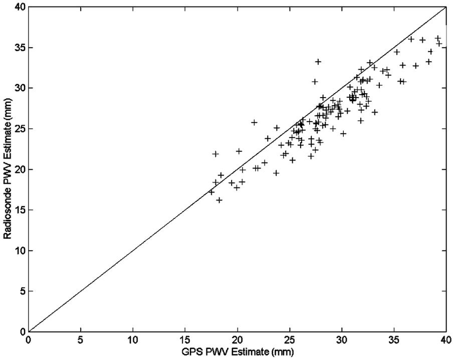
Figure 1. Comparison between radiosonde measured and GPS derived precipitable water.
