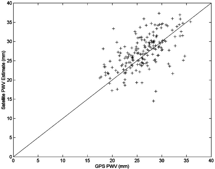
Figure 2. Comparison between GPS-derived and AVHRR satellite-derived estimates of precipitable water based on the Roger and Vermote algorithm (rms error and bias in mm).
