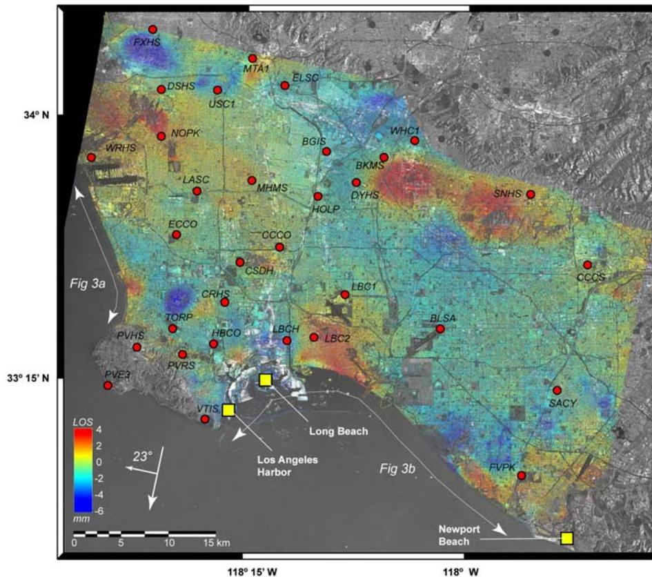
**Figure 1.** Linear line of sight (LOS) velocity from 1992–2000 from ERS-1 descending passes. Continuous GPS stations from the SCIGN network used in our analysis (red circles), NOS tide gauge stations (yellow squares). LOS velocity is with respect to GPS station PVRS. Double-arrow lines along coast indicate areas for the coastal strips plotted in Figure 3. Legend arrow shows ERS LOS azimuth and inclination ( $23^\circ$ ).
